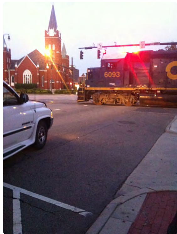
Figure 4.07 – Rail service, once a boon to the Fayetteville economy, frequently interrupts surface roadway travel. All of the rail crossings in downtown are at-grade. The City is working to resolve conflicts by relocating train switching stations, though there are no plans for grade separations. (Image source: Studio Cascade, Inc.)
